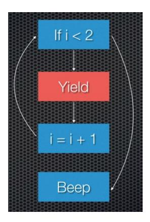
So to unroll the loop, the idea is that there are only two iterations of the loop which the compiler is able to determine.
