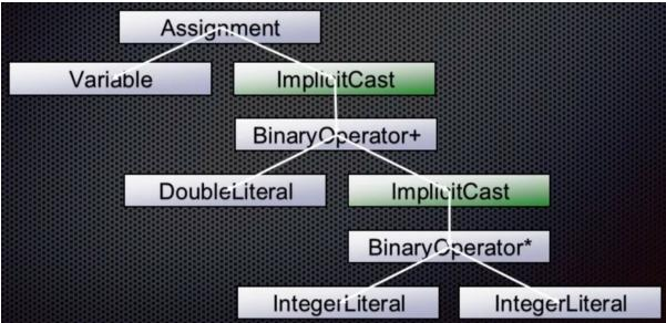
To generate IR, the compiler walks through the above tree, <u>depth first</u>, to get to the leaf nodes. Doing this gets us to the BinaryOperator\* for the multiple on the lower right side of the tree.
